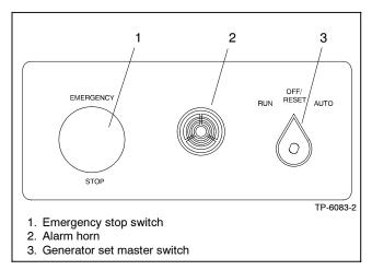
Figure 1-6 Switches and Alarm Horn
